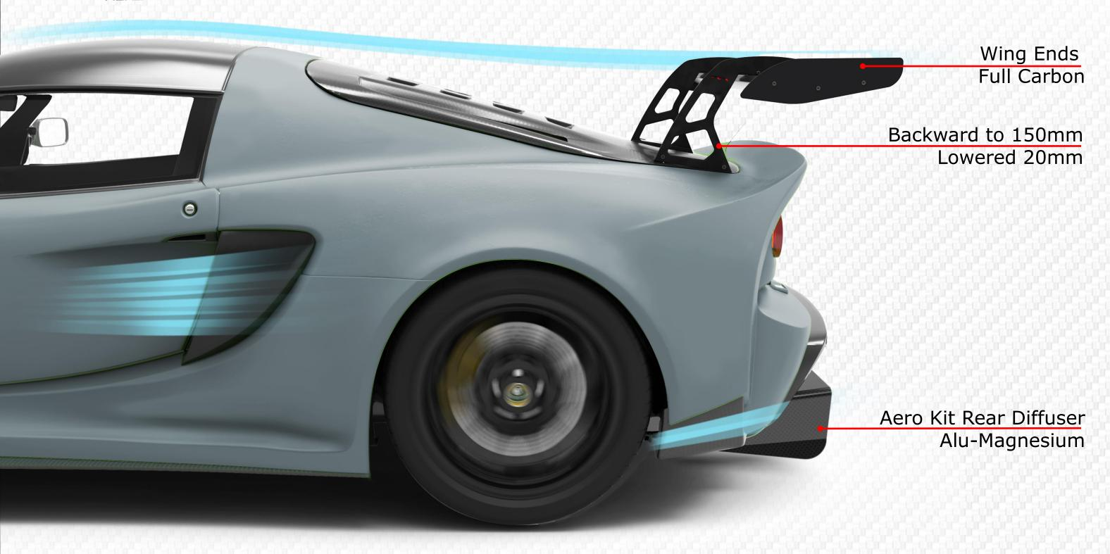
The lower rear diffuser end is perfect with a new designed, significantly larger rear wing, working in synergy to provide 20% more downforce where it matters!
